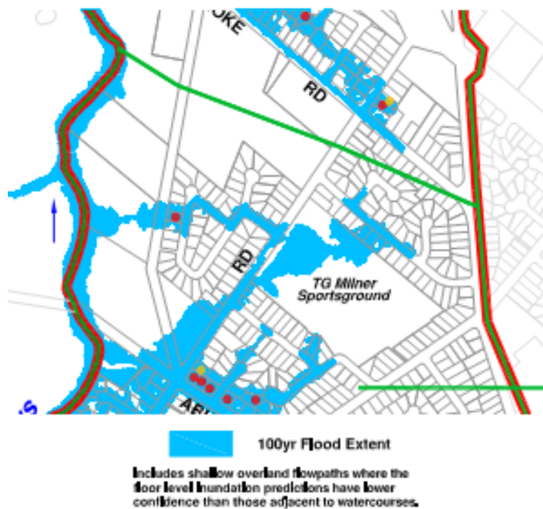
100 Year Flood Extent (Source: Eastwood and Terry Creek Catchment Floodplain Risk Management Study)
